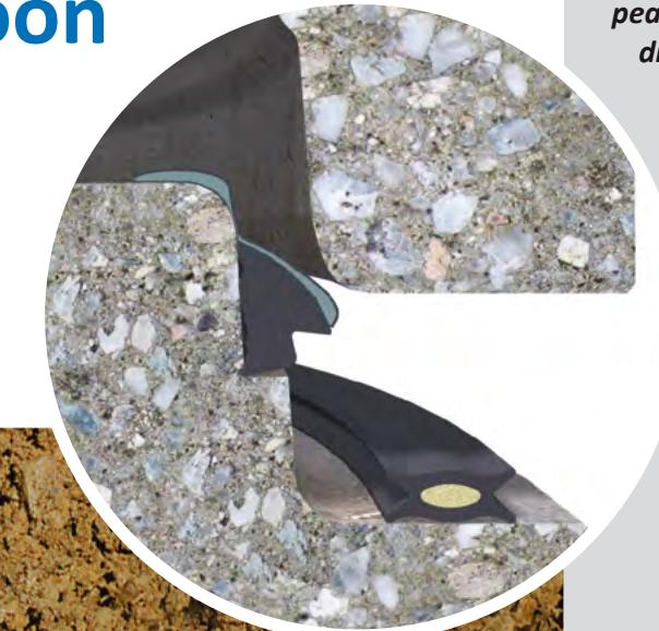
**1.** Pull seal with mantle on top around on the cleaned spigot end, distribute tensioning evenly by repeated pulling at different spots.
