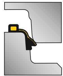
3. Control if the manhole ring is fitting correctly. Make adjustments if necessary.
